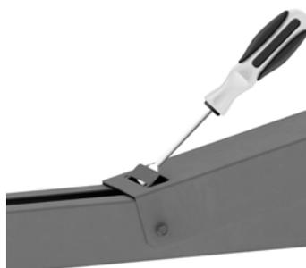
Bend the panel stop in an angle of 90° using a screwdriver.
